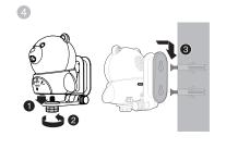
Place the baby unit on the wall mount bracket. Tighten the screw into the threaded socket at the bottom to secure the baby unit. Align the holes on the wall mount bracket with the screws on the wall, and slide the wall mount bracket down until it locks into place.
